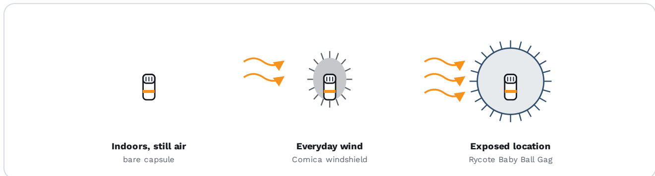
Fig. 6.1 Level of protection according to wind exposure.
